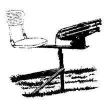
Be careful when cocking the thrower arm or placing a target on it. It can deliver a very powerful blow if released.
